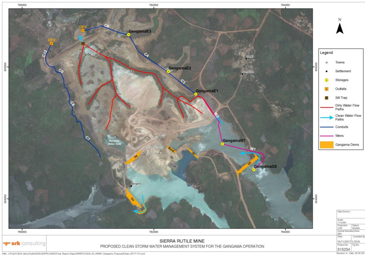
Figure 53. Proposed storm water management system for Gangama dry mine (source SRK 2018 Surface Water Specialist study)
