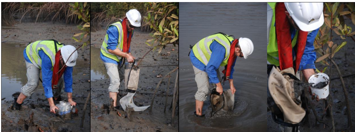
Figure 7. Collection of intertidal macrofauna samples with a hand held corer (1), transfer to a 1 mm mesh bag (2), rinsing to remove fine sediment (3) and transferring the residual material to a sample jar (4).
