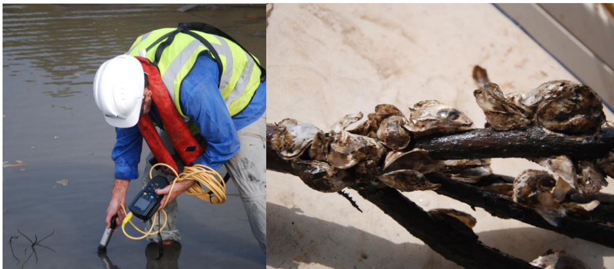
Figure 5. Measuring water quality parameters (temperature, salinity, DO and pH) using a HachHQ40d water quality meter (left) and mangrove oysters used for biomonitoring (right).
