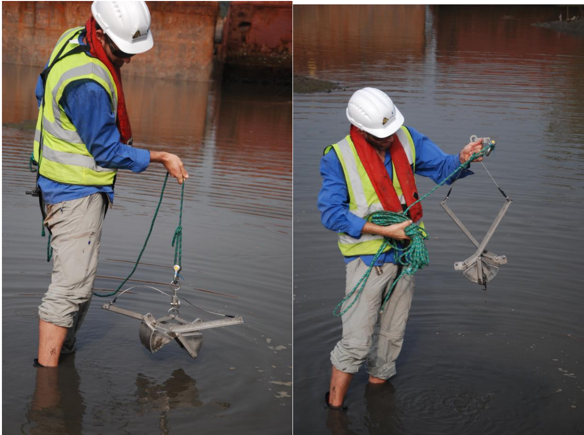
Figure 6. Sub-tidal macrofauna and sediment samples were collected using a Van Veen grab. Typically this was done in the channel from a boat but the action of the grab is demonstrated here on the edge of the bank.
