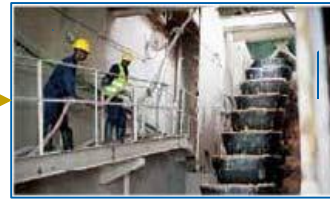
Bucket ladder Dredge designed to dig at a rate of 1,000 tonnes per hour
