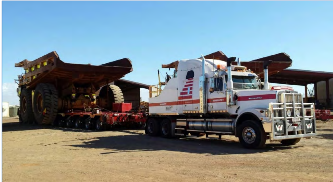
Figure 4-3: Example SME transport (Image Sourced from Mammoet Australia)
