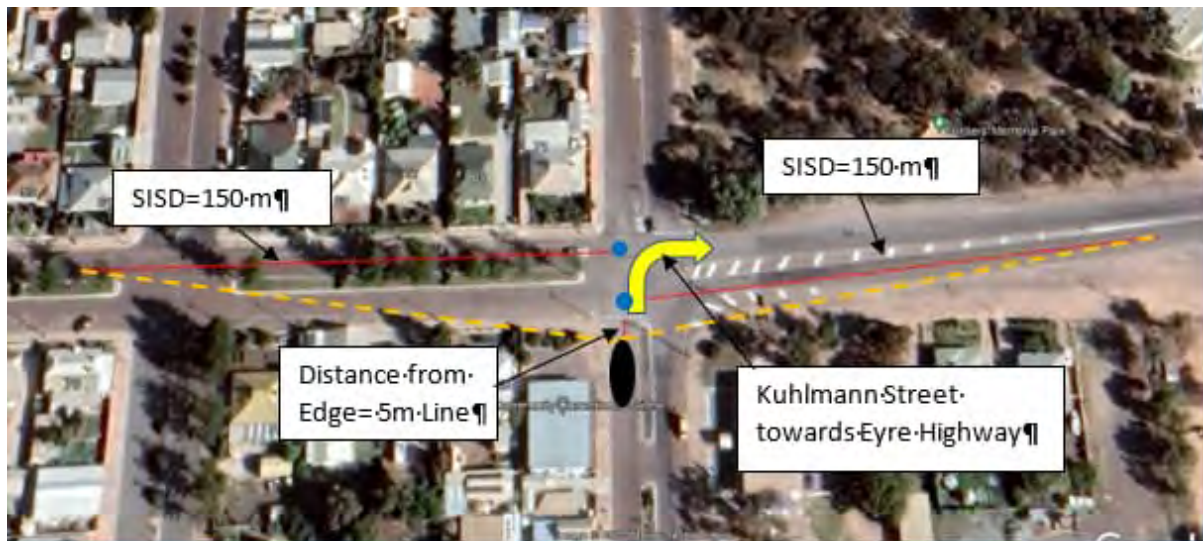
Figure D-2: SISD Check for Right Turn from Kuhlmann Street onto Eyre Highway
