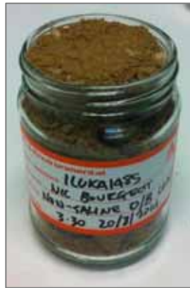
Figure 4: Example of composite sample - NSOB Composite prior to sealing and dispatch.
