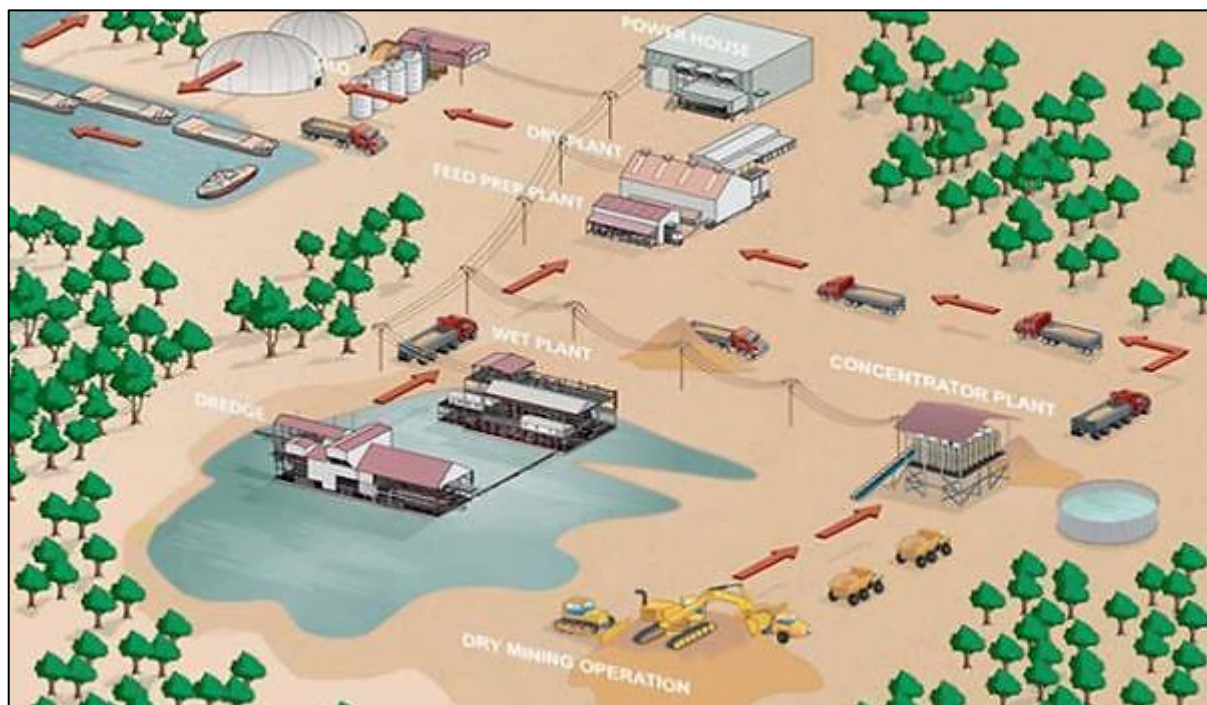
Figure 1.3: Simplified mining operations and processes
