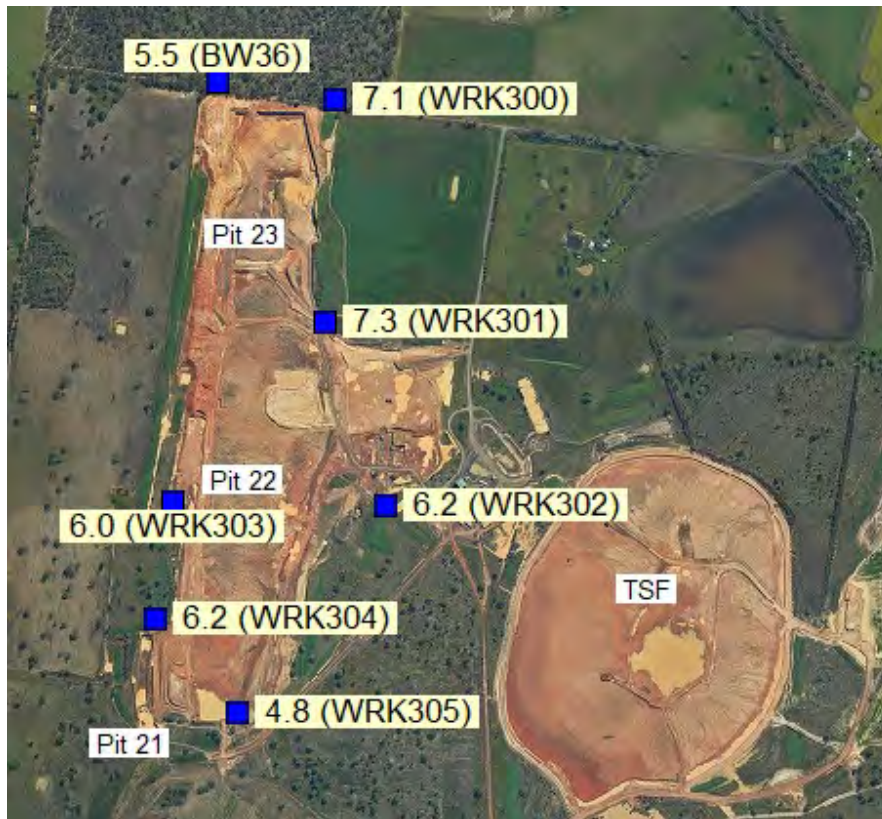
Figure 3.8 Locations and latest (2018) pH measurements of bores surrounding Pit 23
