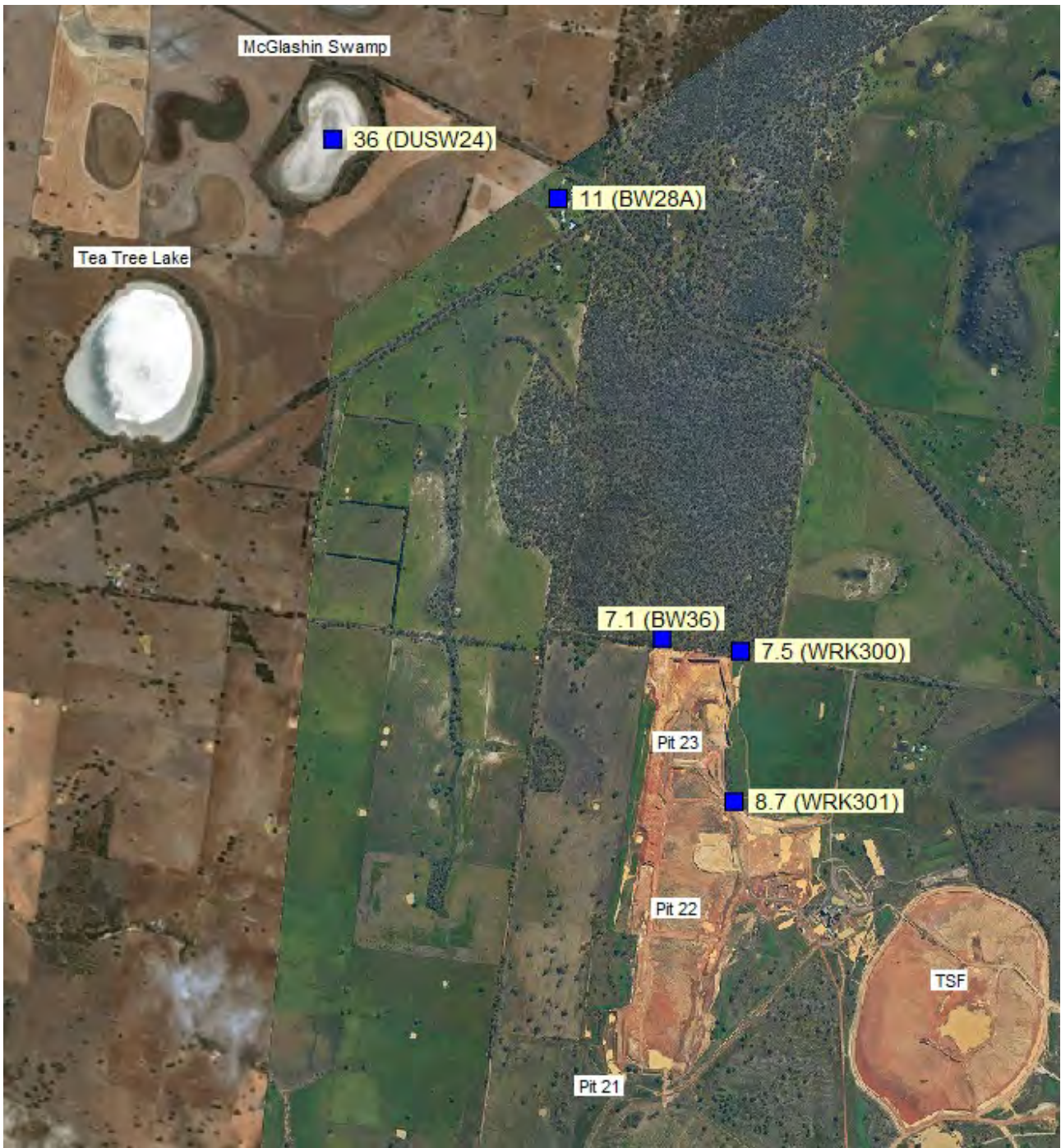
Figure 3.15 Locations and latest (2018) \text{Cl}:\text{SO}_4 measurements of bores in or near the groundwater flow path from Pit 23 and at McGlashin Swamp (DUSW24)
