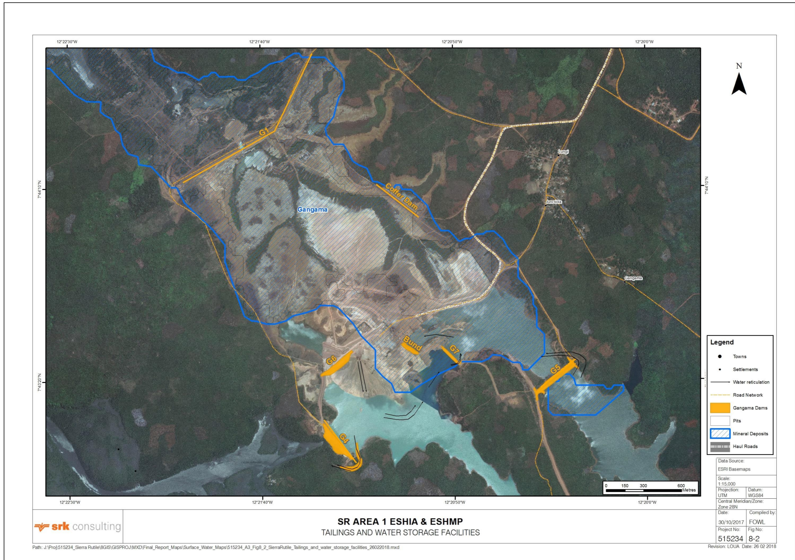
Figure 8-2: Gangama DM2 tailings and water storage facilities
