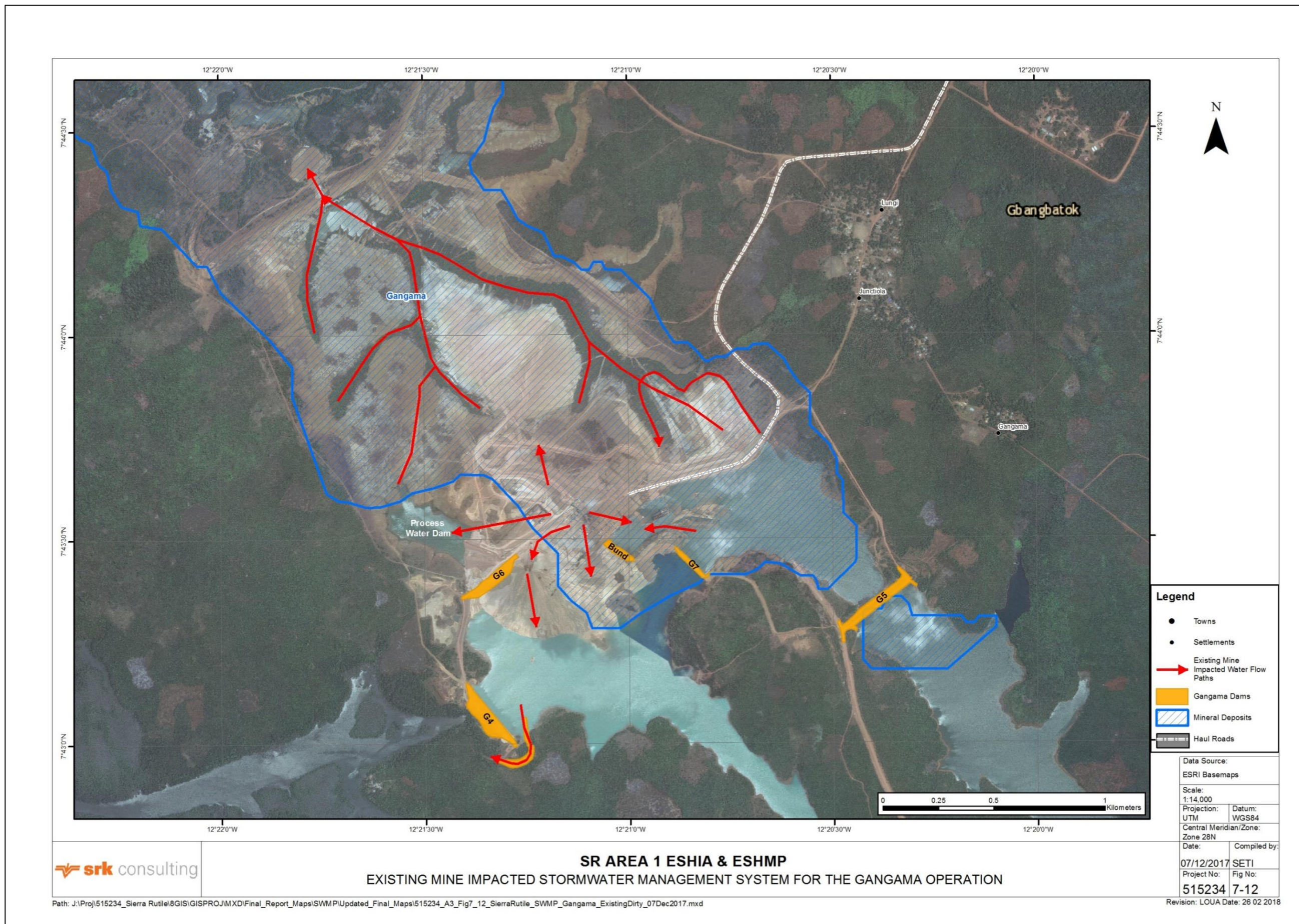
Figure 7-12: Existing mine impacted stormwater management system at the Gangama operation
