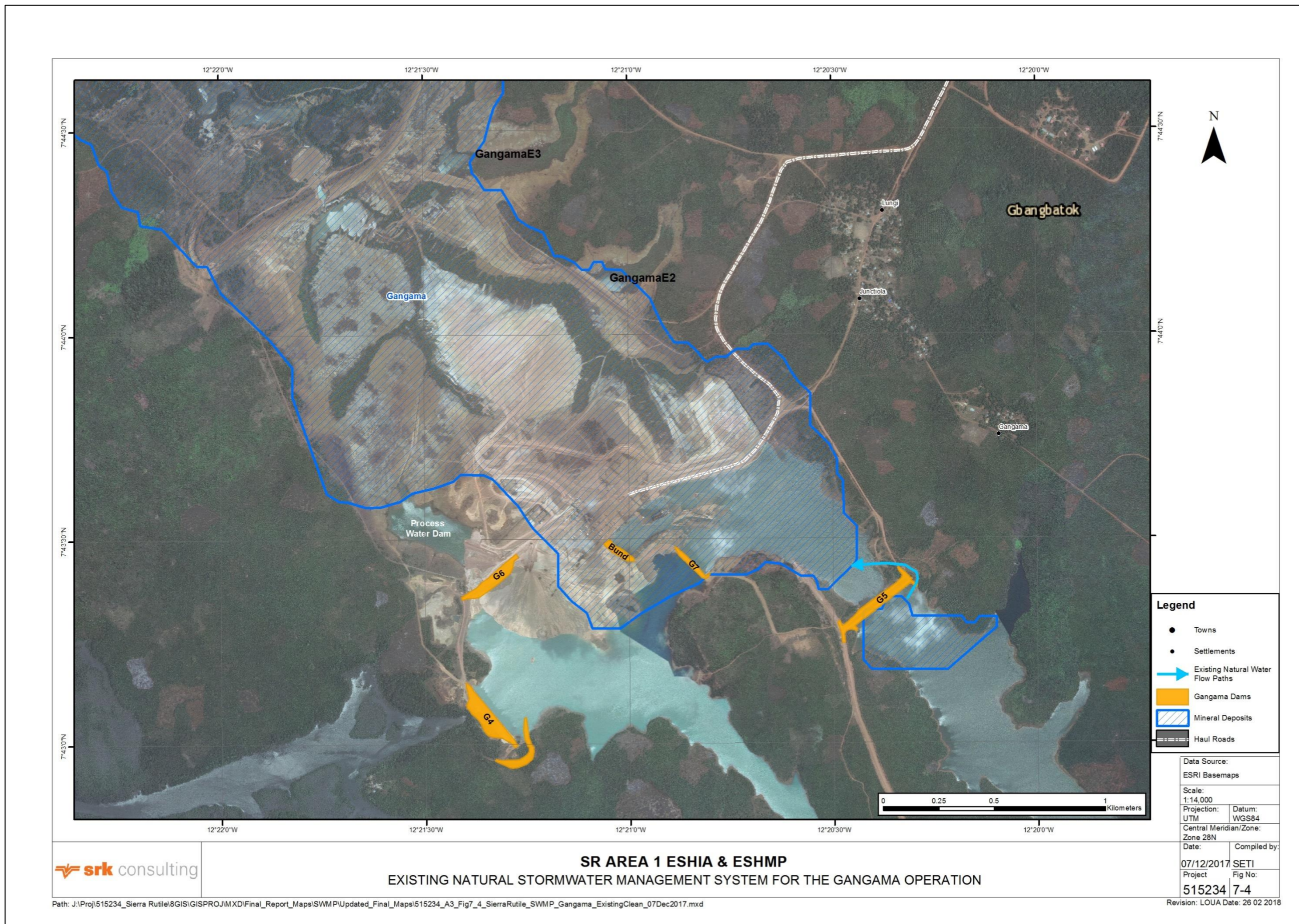
Figure 7-4: Existing natural stormwater management system at Gangama operation
