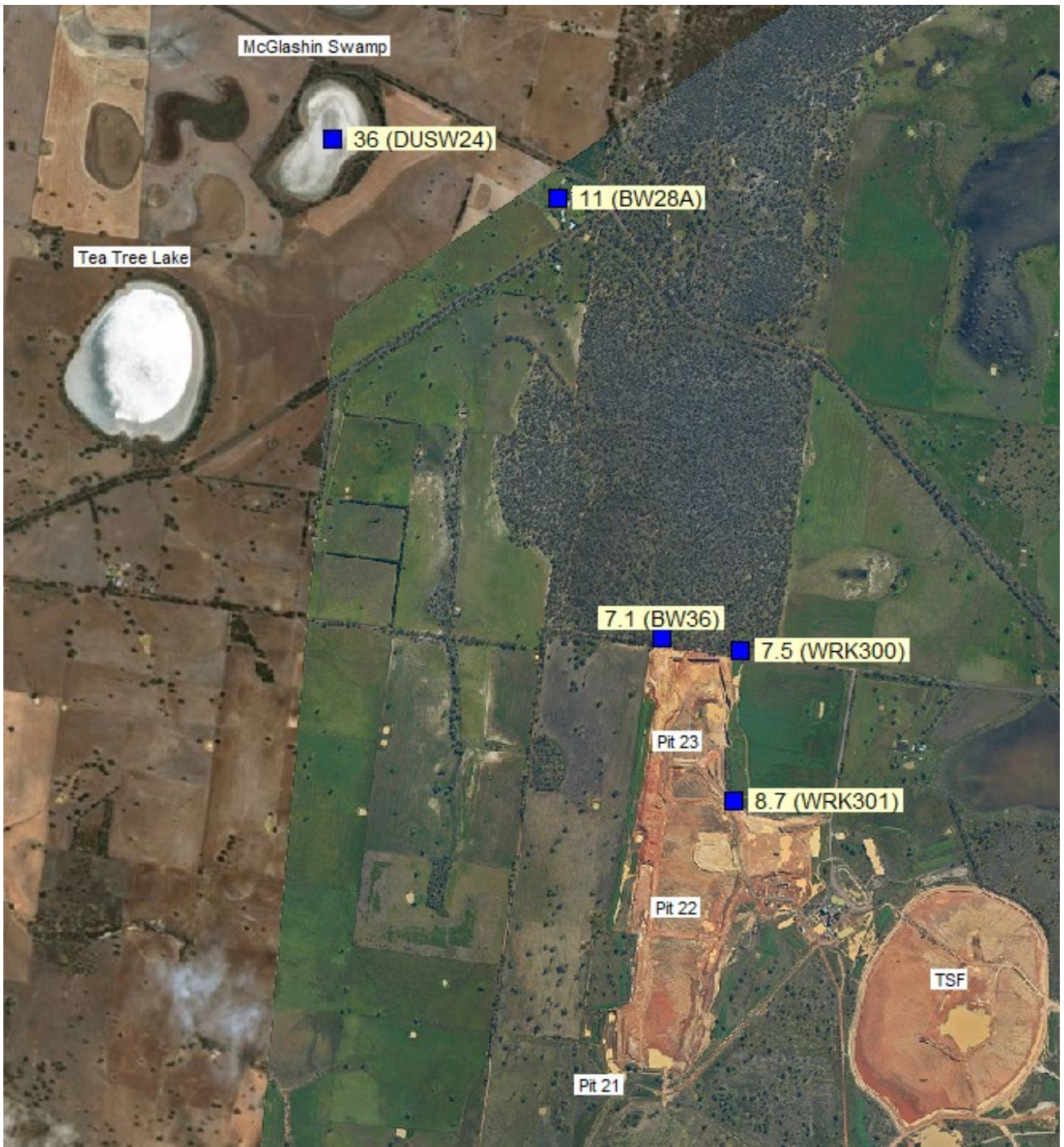
Figure 3.15 Locations and latest (2018) Cl:SO 4 measurements of bores in or near the groundwater flow path from Pit 23 and at McGlashin Swamp (DUSW24)
