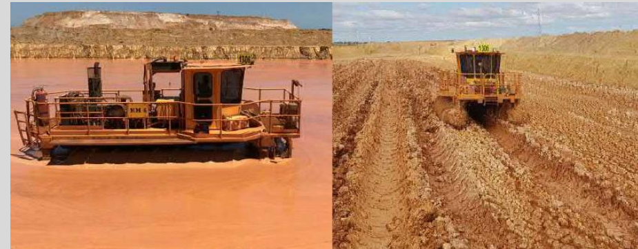
Amphiroller in the Accelerated Mechanical Consolidation (AMC) cell
