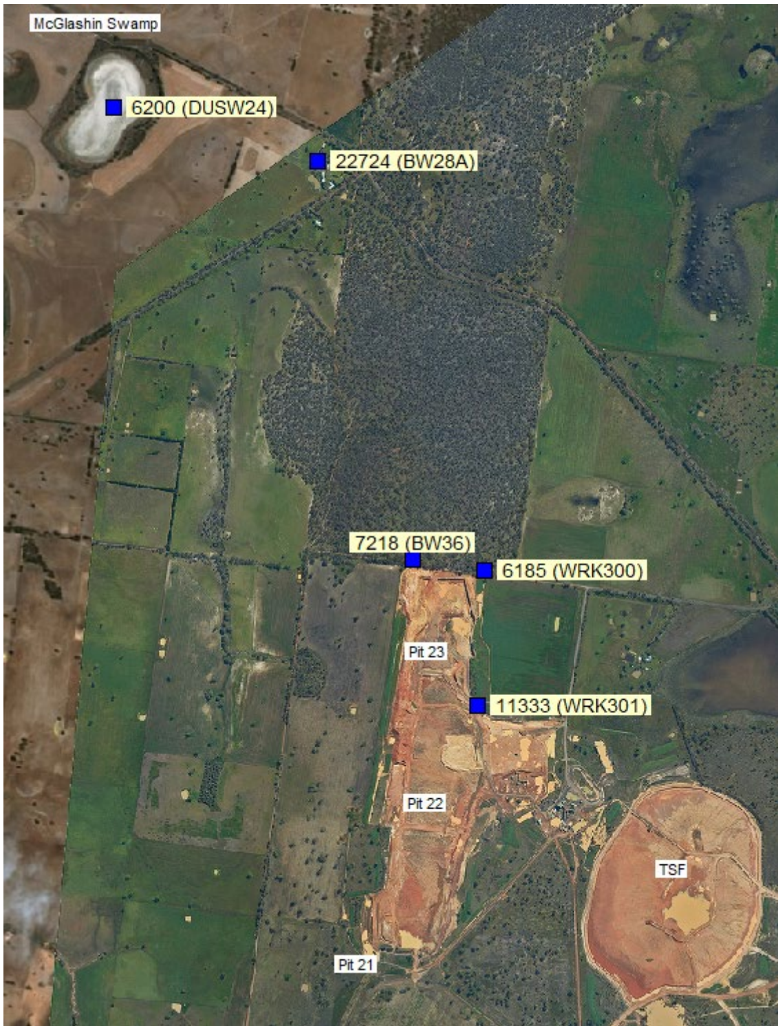
Figure 3.5 Locations and latest (2018) electrical conductivity measurements ( \mu\text{S}/\text{cm} ) of bores in or near the groundwater flow path from Pit 23 and at McGlashin Swamp (DUSW24)
