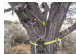
Sap flow measurement is used to investigate whether hydraulic distribution is used to redistribute water via root system into deeper soil layers during dry seasons.
