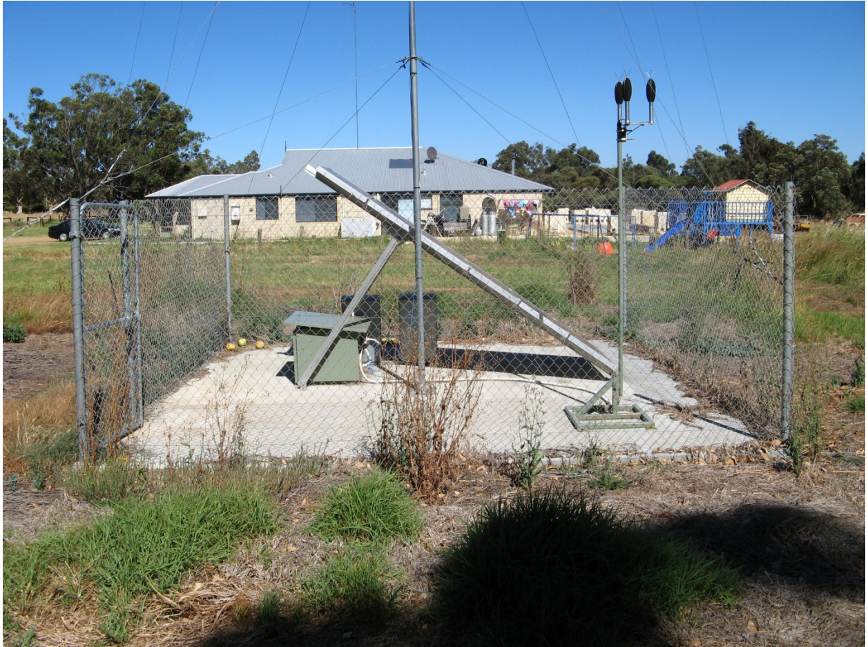
Figure 8. Example of the directional sound level meters (DSLM) used at Tutunup South Mine.
